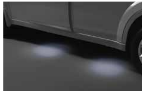
85 Puddle Lamps H471SAJ000 Located at the bottom of the vehicle and activates when door is opened.
