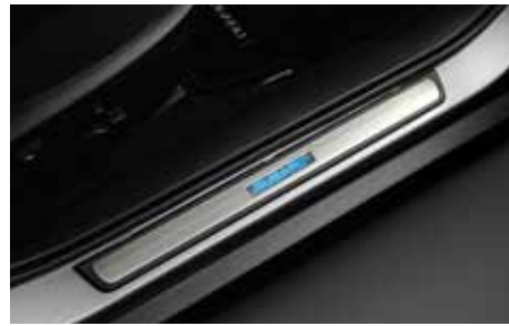
84 LED Side Sill Plate H1010AJ000 High-grade stainless-steel sill plate equipped with a SUBARU logo light.
