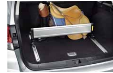
45 Luggage Partition L0010AJ010 Partition off the cargo space when used in combination with Rail & Hook Kit.
