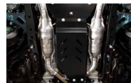
42 Transmission Under Guard
