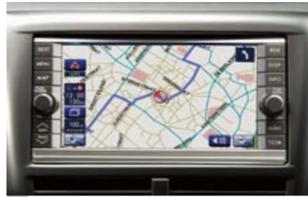
86 DVD-Navigation kit (L.H.D., R.H.D.) H001EFG001, H001EFG011 Exclusive design, user-friendly operation with touch screen and easy destination input. Includes radio, CD player, and DVD player. Bluetooth handsfree pre-arranged *Map DVD is not included
