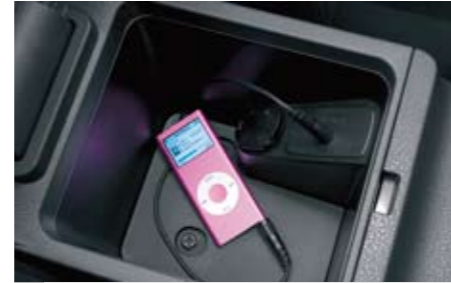
83 AUX outlet kit H6210FG000 A 3.5 mm auxiliary stereo mini-pin jack socket that allows you to listen to the sounds from portable music players. Now you can enjoy your own music through the car speakers. *For factory installed 1CD audio.
