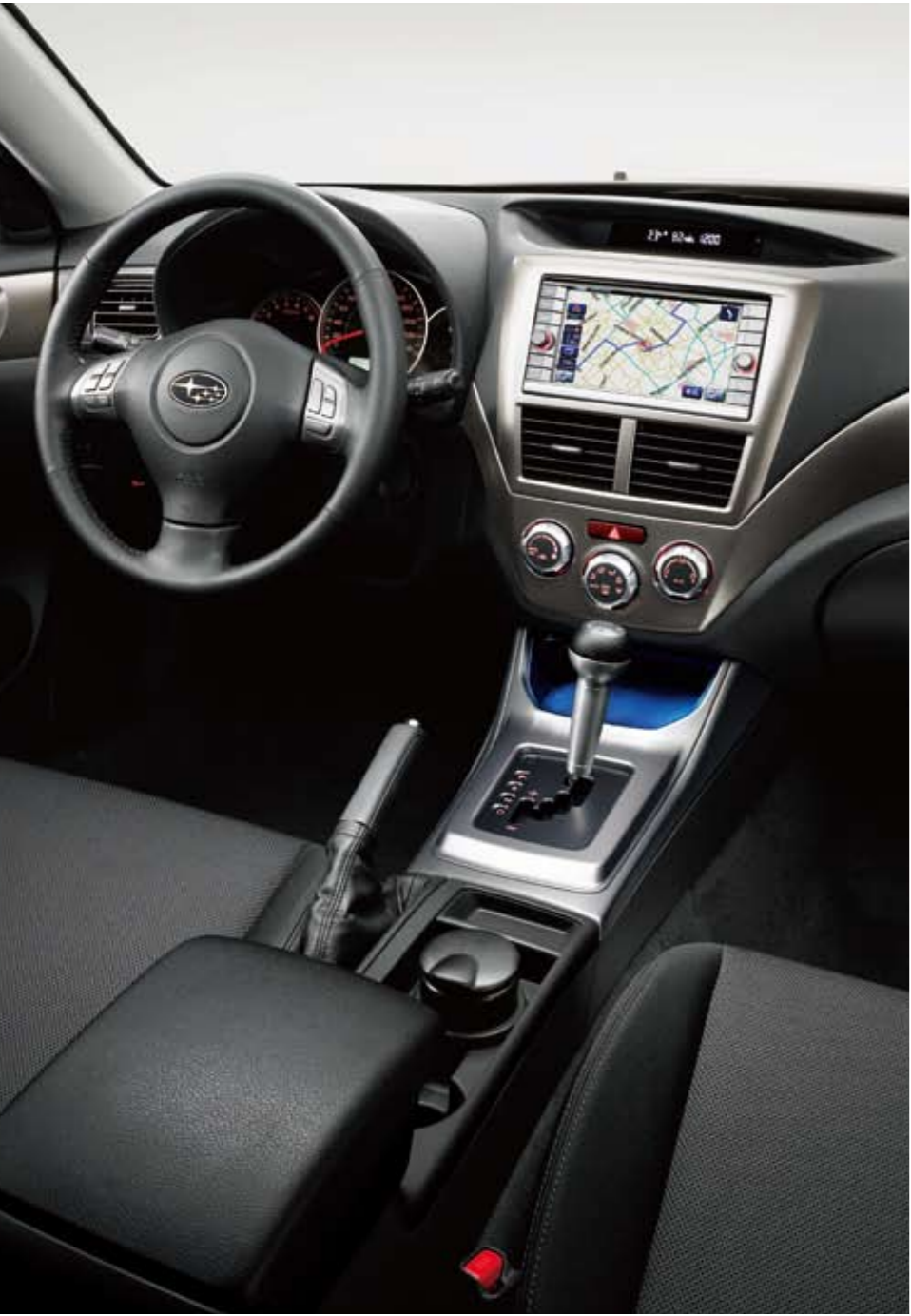
Image: vehicle is presented with Aluminium shift knob, round type ashtray, Dual console box, Navigation kit.
