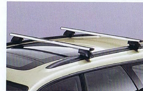
25 Carrier base E361EAG100 W Perfectly fitting stylish base for carrier attachments.
