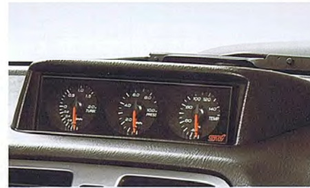
101 STI, Sports gauge pack (L.H.D.) H5010FE500 W Turbo boost, oil temp, oil pressure gauge.
