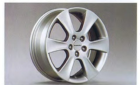
32 Alloy wheel (16 inch) SECWFE4000 E 6.5"x16" offset 55 Tyre size: 205/55 R16, 205/50 R16(snow)
