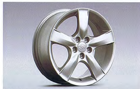
30 Alloy wheel (16 inch) 28111FE310 W 6.5"x16" offset 55 Tyre size: 205/55 R16, 205/50 R16(snow)
