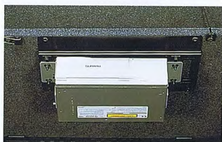
95 CD changer bracket (Wagon) H6210FE900 W Attachment required to mount CD changer or Navi unit.
