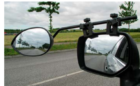
10 Caravan Mirrors (Set of 2) HF05100S Aerodynamic caravan mirrors attached to the original rear view mirror with two clamps. The mirror head is by dripping format which minimizes air resistance and provides an almost vibration free mirror. Mirror size: 20,5x12,5 cm. Convex mirror glass. Long arms to be useful with wider caravans. Supplied with handy storage bag. Set of 2.
