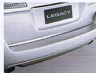
52. Rear gate end moulding (Wagon)
